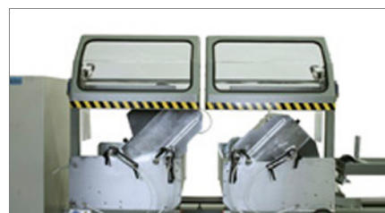
Tilting of the moving cutting heads
