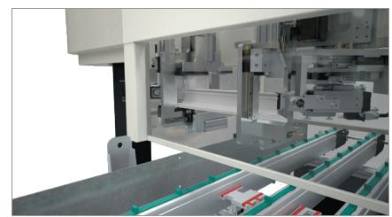
Milling on the two profile ends at the same time
