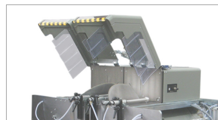
Tilting of the moving cutting heads
