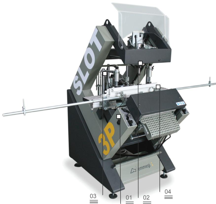
Automatic water slot milling machine also for drilling ventilation holes on PVC profiles. The machine features 3 cutter heads with pneumatic feed and traversing on recirculating ball slideway packs which can be selected independently. The cutter heads are provided with memorizable adjustments through 6 stops on the stroke and 6 stops for head positioning. Tilting of the cutter heads is adjustable thanks to the angular references.
