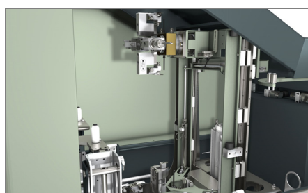
Cleaning module with 2 interpolated axes 03
