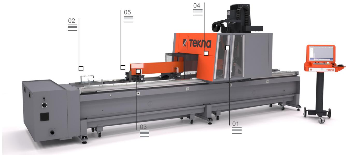
Mobile gantry CNC 4-axis machining centre, designed for drilling, milling and threading at any angle from -90° to +90° on bars or pieces in aluminium, PVC, light alloys in general and steel. The mobile part of the machine mainly consists of a gantry equipped with precision motorisation rack. The 8.5 kW electrospindle with ISO 30 tool connection is able to perform even heavy-duty machining with excellent, rapid and accurate results.
